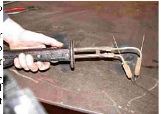
Shows the torch and the position of the two tungstens
