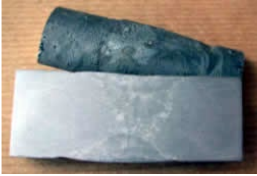
Shows macro of completed weld in a 12mm steel bar
